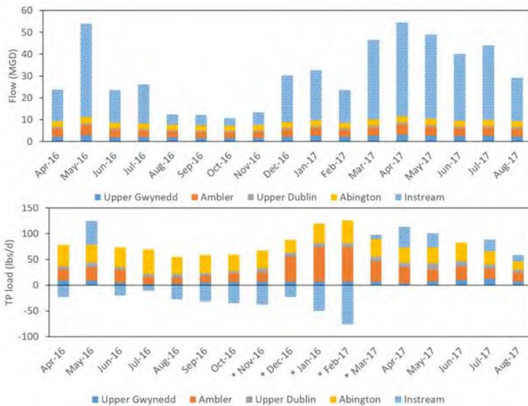
Figure 11 - Apportionment of Flow (upper) and Total Phosphorus Load (lower) at Fort Washington for Both Storm and Base Flow. Note that Upper Gwynedd loads are estimated for 5-months (indicated with *). Instream discharge and TP load are solved by difference.
