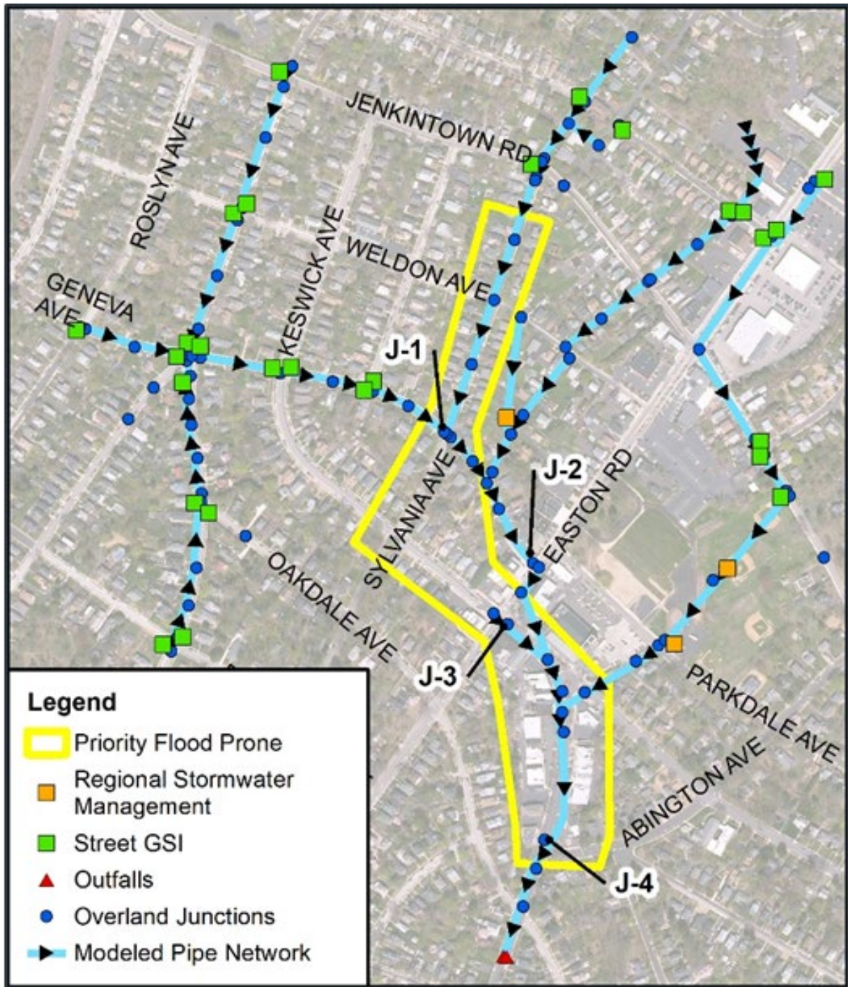
Figure 3-6: ALTERNATIVE 4 – REGIONAL STORMWATER BASIN WITH GSI
